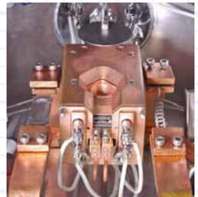
4 pocket e-beam source & 2 thermal resistance sources [boat & coil].
