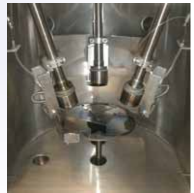
Chamber with an array of three 1" magnetron guns with pneumatic shutters, thickness sensor & rotating stage.
