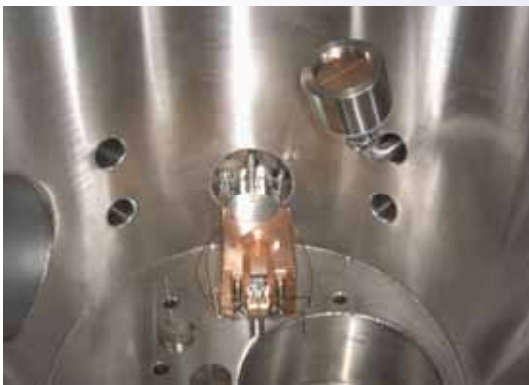
Full front door opening D shaped box chamber fitted with one 4 pocket e-beam source and one fixed 2" magnetron gun.
