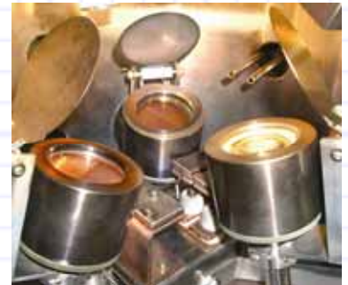
Three shuttered 2" magnetron guns and 2 thermal resistance sources.
