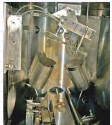
E-beam, ion beam, thermal resistance and magnetron sputtering sources with shields & shutters, and rotating substrate stage with full axis radial tilt.
