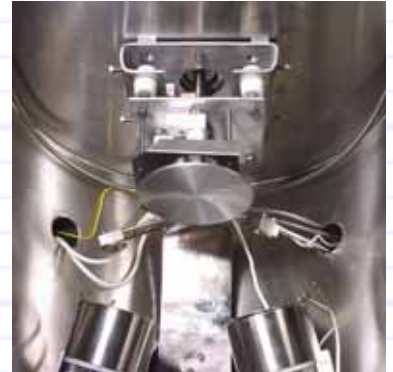
Two 2" magnetron guns with quartz thickness sensors and a heated substrate stage with variable axis rotation.
